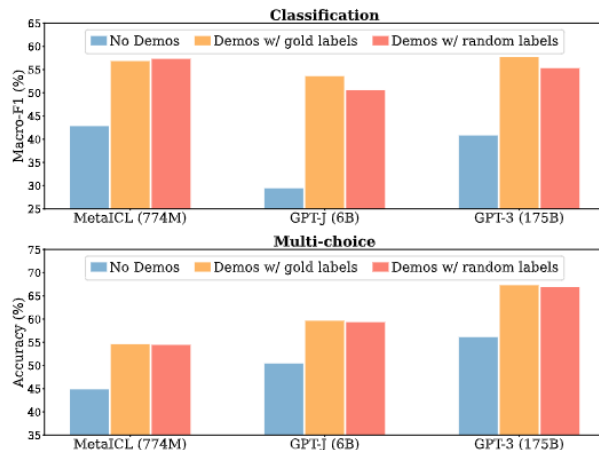
Figure 1: Results in classification (top) and multi-choice tasks (bottom), using three LMs with varying size. Reported on six datasets on which GPT-3 is evaluated; the channel method is used. See Section 4 for the full results. In-context learning performance drops only marginally when labels in the demonstrations are replaced by random labels.
